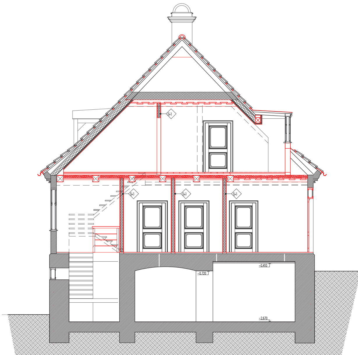
The drawing of the building reconstruction – on the edge – the changed coverings among the current bearing structures and the ceiling boards which are insulated. 16
